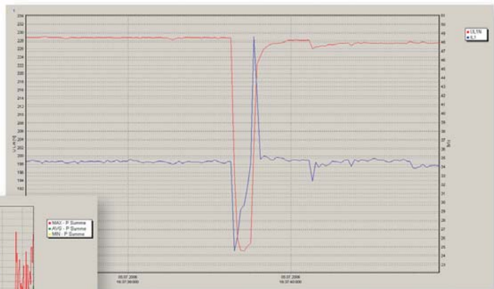
Example of a trigger event, one phase voltage and current.
